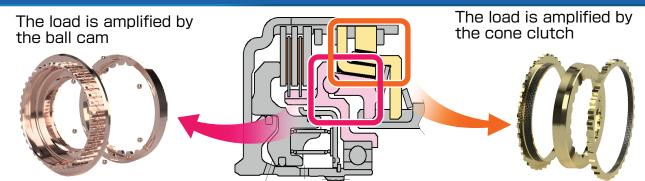
The load amplified by the ball cam is further amplified by the cone clutch. The flood control is greatly reduced by the amount that the load is amplified.
